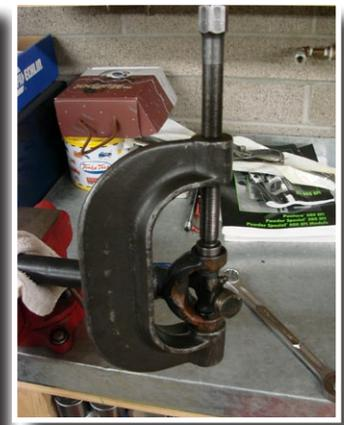
With the clamp we have we just tighten it down and the u-joint gets pressed towards the opposing side of the yoke. If you don't have access to one of these clamps used to press u-joints out you can use a brass drift or a hardened socket (like an impact socket) to drive the old one out. Once the u-joint has slipped out of the yoke you just need to remove one of the needle bearing caps and the u-joint can be removed from the yoke.
