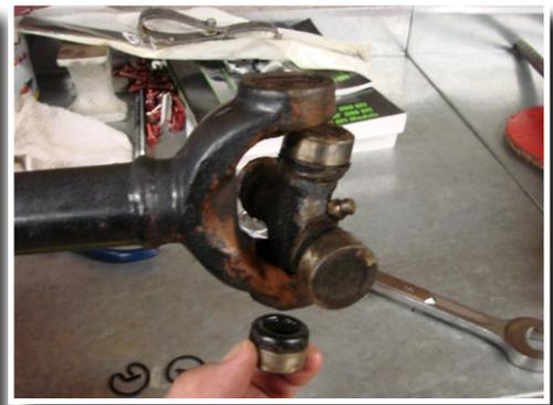
Once the old joint has been removed it is good to clean out the yoke and slightly lube it to assist in installing the new one.
